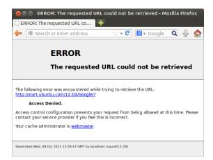
What caused the Access Denied error? We need to find out how Squid access control works. It's defined in the Squid configuration file, /etc/squid3/squid.conf, by the following lines:
